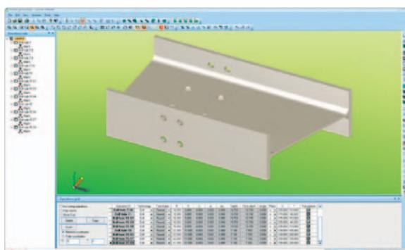
Once the design process is completed, the user can simulate the head movement of the machine, the beam or tube movement, and the machining operations of
